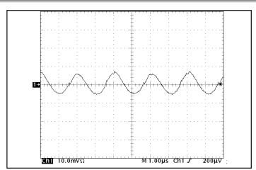
Figure 13: Input Terminal Ripple Current, ic, at full rated output current and nominal input voltage with 10  $\mu H$  source impedance and 47  $\mu F$  electrolytic capacitor (500 mA/div). See Figure 12.
