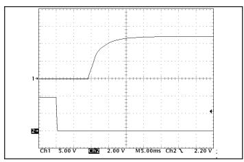
Figure 9: Turn-on transient at half load (resistive load) and 3mF output capacitance (5 ms/div). Input voltage pre-applied. Ch 1: Vout (5 V/div). Ch 2: ON/OFF input (2 V/div).
