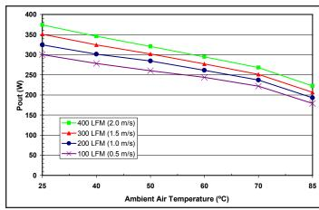
Figure 8: Maximum output power derating curves vs. ambient air temperature for airflow rates of 100 LFM through 400 LFM with air flowing from input to output (nominal input voltage).
