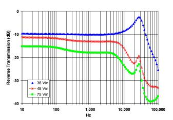
Figure 20: Magnitude of incremental reverse transmission (RT = Iin/Iout) for minimum, nominal, and maximum input voltage at full rated power.
