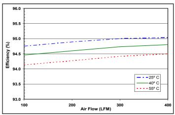
Figure 3: Efficiency at nominal output voltage and 60 % rated power vs. airflow rate for ambient air temperatures of 25, 40, and 55 °C (nominal input voltage).
