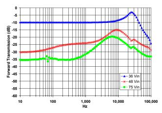
Figure 19: Magnitude of incremental forward transmission (FT = Vout/Vin) for minimum, nominal, and maximum input voltage at full rated power.
