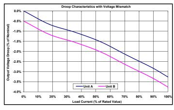
Figure F: Example of Droop Characteristic with Output Voltage Mismatch.
