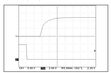
Figure 10: Turn-on transient at zero load and 3 mF output capacitance (5 ms/ div). Input voltage pre-applied. Ch 1: Vout (5 V/div). Ch 2: ON/OFF input (2 V/ div).
