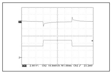
Figure 11: Output voltage response to step-change in load current (50%-75%-50% of Iout(max);  $dI/dt = 0.1 A/\mu s$ ). Load cap: 100  $\mu F$ , electrolytic cap, 15 uFtantalum cap, and 1 µF ceramic cap. Ch 1: Vout (2 V/div), Ch 2: Iout (10 A/div).
