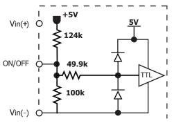
Figure B: Internal ON/OFF pin circuitry
