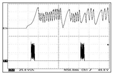
Figure 17: Load current (25 A/div) as a function of time when the converter attempts to turn on into a 1 m $\Omega$  short circuit. Top trace (500 us/div) is an expansion of the on-time portion of the bottom trace
