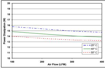
Figure 4: Power dissipation at nominal output voltage and 60 % rated power vs. airflow rate for ambient air temperatures of 25, 40, and 55 °C (nominal input voltage).
