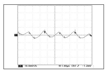
Figure 14: Input reflected ripple current, is, through a 10  $\mu H$  source inductor, using a 47 µF electrolytic input capacitor (20 mA/div). See Figure 12.
